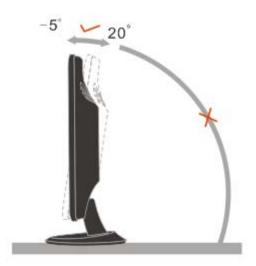
NOTE: Do not touch the LCD screen when you change the angle. It may cause damage or break the LCD screen. Cable Connections On Back of Monitor and Computer
